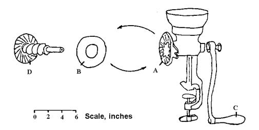
Hand operated grain huller: A) stationary disk, B) rubber disk, C) handle and D) rotating disk with auger. Remove stationary disk and replace with rubber-faced disk.
